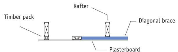
Alternatively the diagonal brace may be replaced within the sloping ceiling area by a plywood diaphragm fixed between the relevant rafter members.
