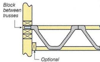
Intermediate Simple Span
