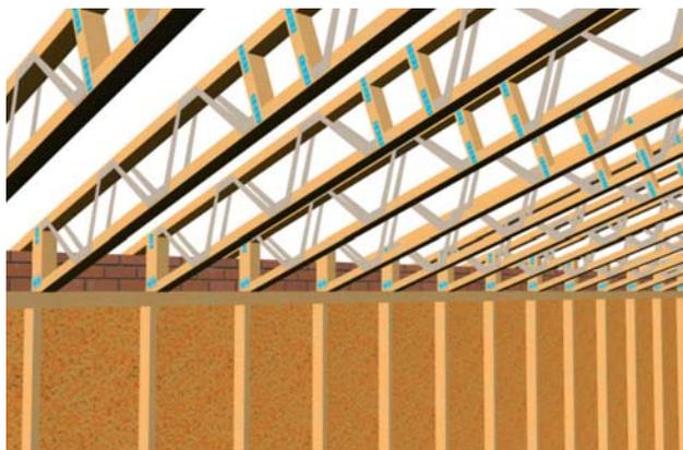
Open web joists can be used for pitched roofs.
