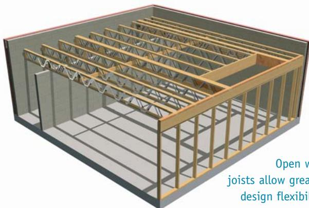
Open web joists allow greater design flexibility
