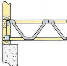
Bottom Chord Bearing - Masonry Wall
